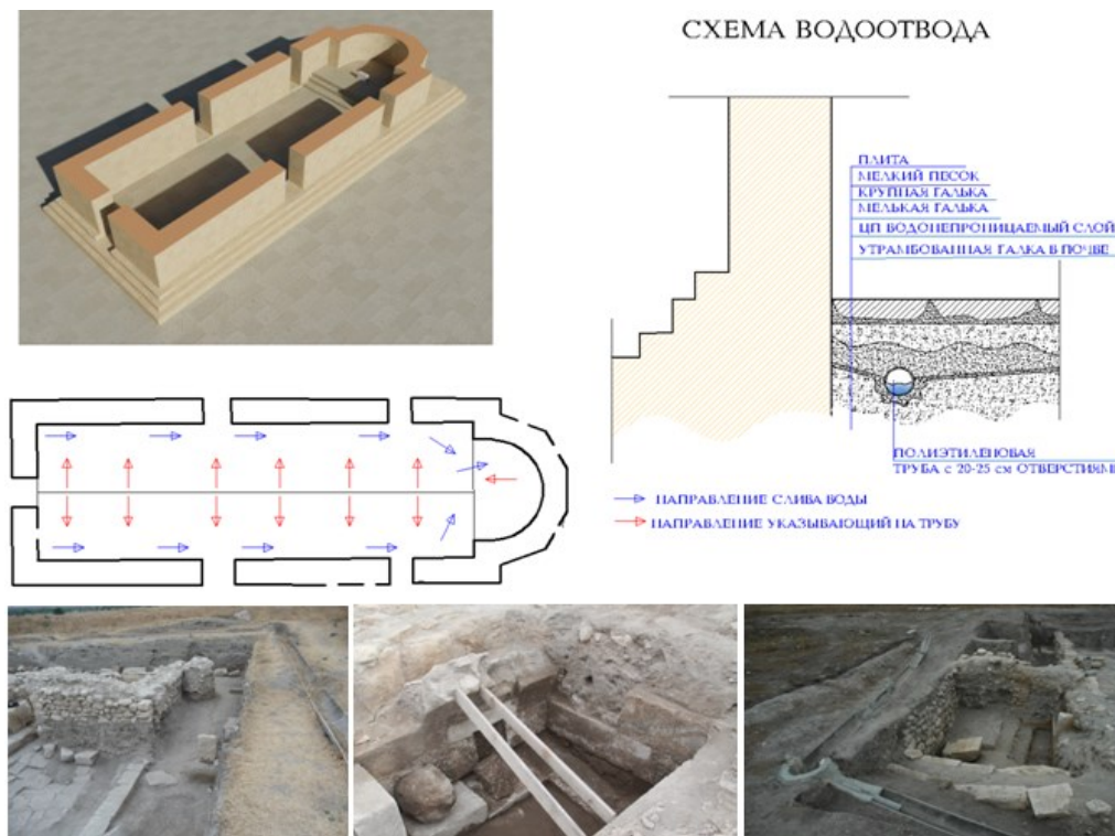
Fig. 4. The inner and outer drainage system of the basilic church of Tigranakert. Photo of the author
